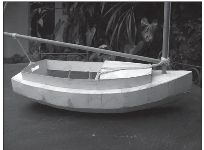
I built a scale model in cardboard to see the design and refine the shape.
