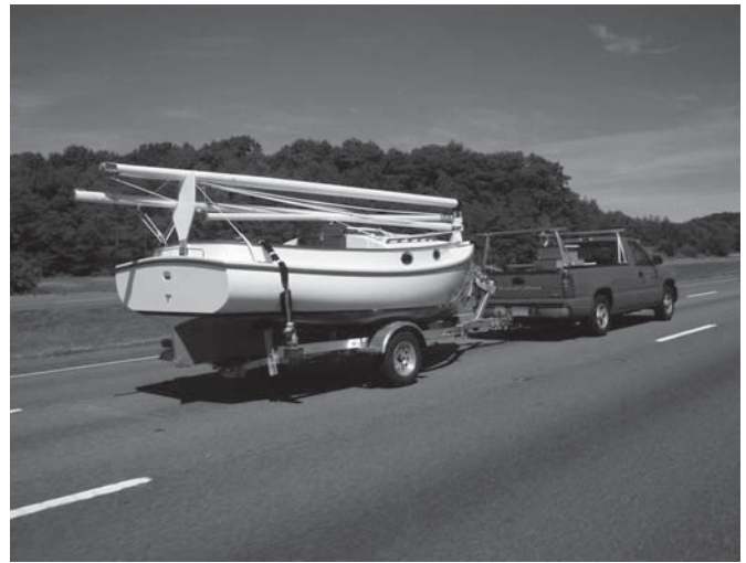
A Marshall Sanderling traveling on a highway with the mast tabernacle in the down position.
