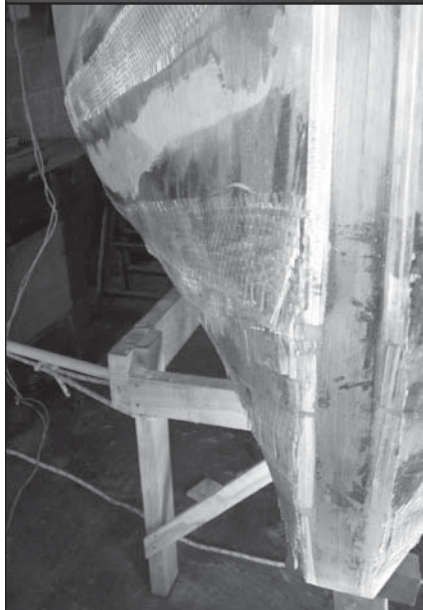
To achieve the fine entry, with the compound curves, I had to use several, narrow, fitted planks to get the shape I wanted.
