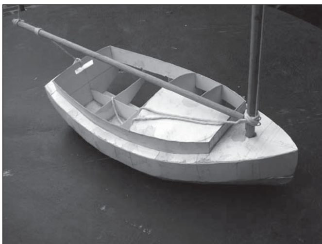
To achieve the fine entry, with the compound curves, I had to use several, narrow, fitted planks to get the shape I wanted.
