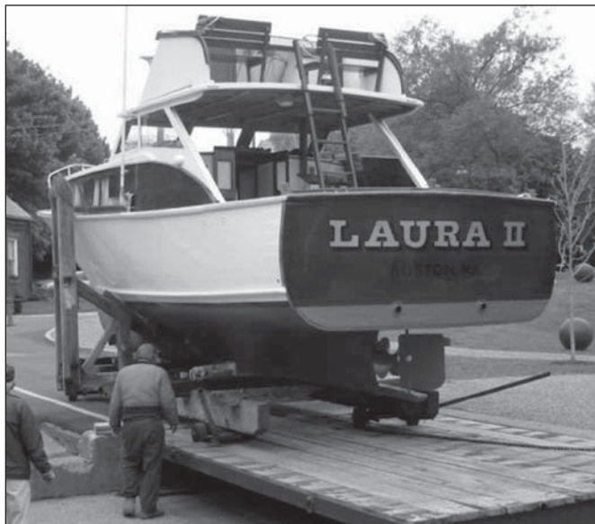
Removable wheel sets placed at each corner of the cradle to facilitate moving boats in the yard.
