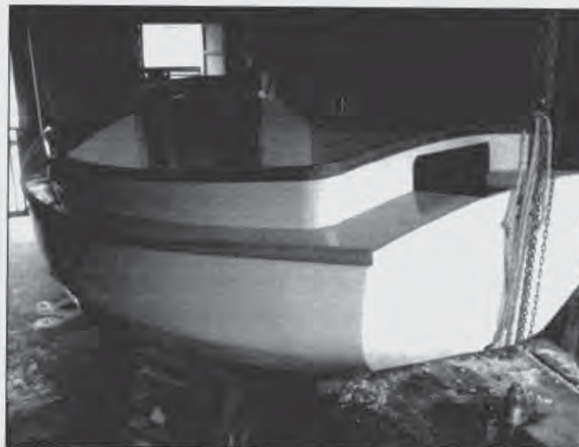
Lifted stern for cradle placement to keep boat from rocking while working inside.
