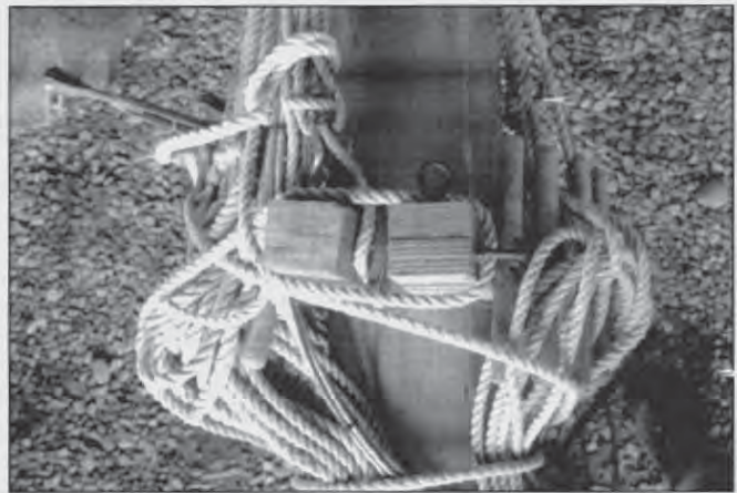
Threaded rod, nut, and screw eyes for attachment.
