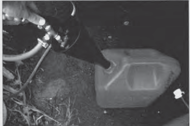
The siphon in use at the can end.
