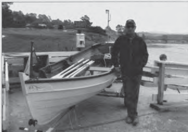
Penobscot row boat constructed in wood epoxy with plywood lapstrake planking next to the builder.
