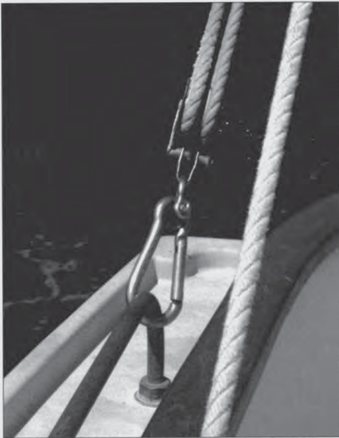
Carabineer attached to the lower block and traveler.
