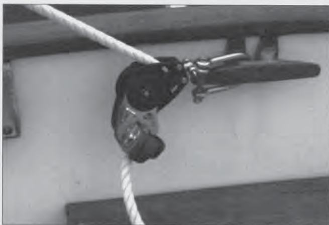
Mainsheet block and cam cleat assembly installed on the existing horn cleat.
