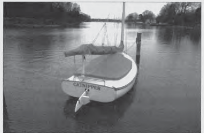
Catnipper , a 1998 Fenwick Williams 16 ft. Lowery build catboat. Note again the outboard motor bracket on the rudder. Also, great canvas work on the cockpit cover.
