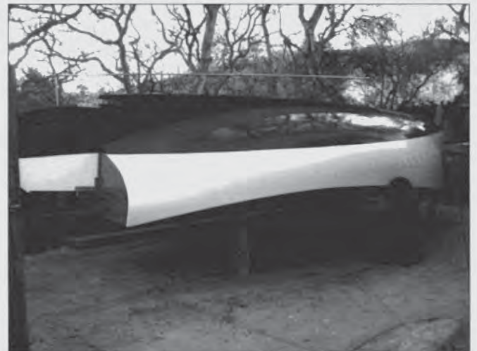
Hull with skeg, rudder attached, painted and ready to be turned over.
