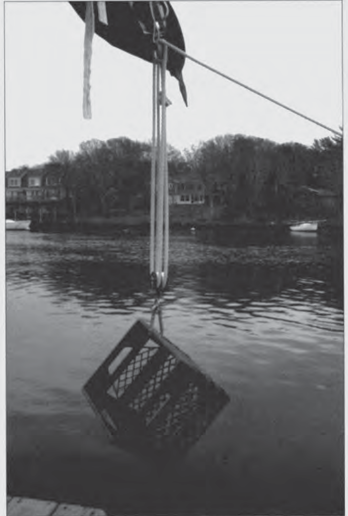
Figure 2 – An example of how the man-overboard tackle is used.
