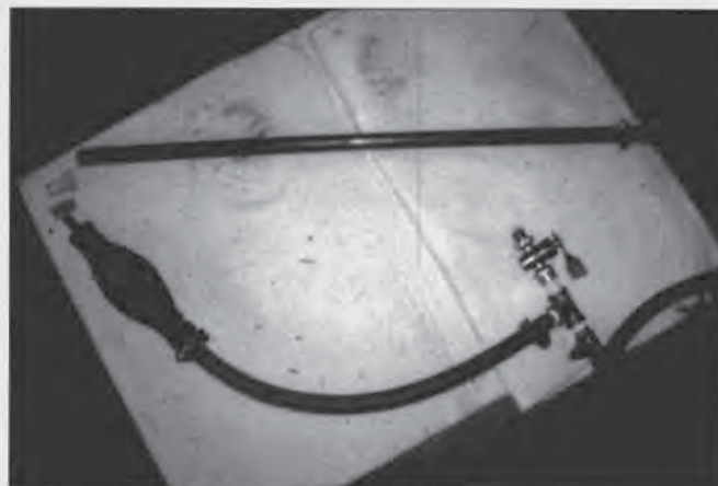
The assembled siphon.
