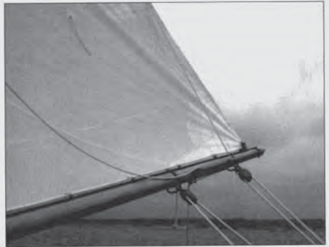
Shown here are the mainsheet and blocks, and the lazy jack fitting.
