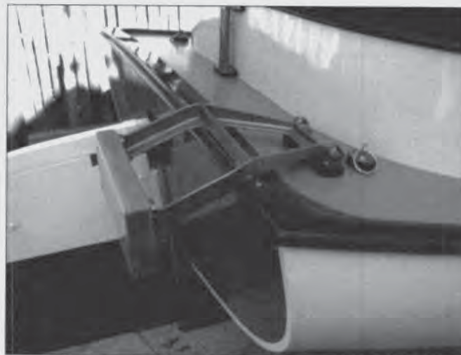
The outboard bracket chosen is not too unsightly. When I want to sail without an engine, it and the bracket are easily removed.
