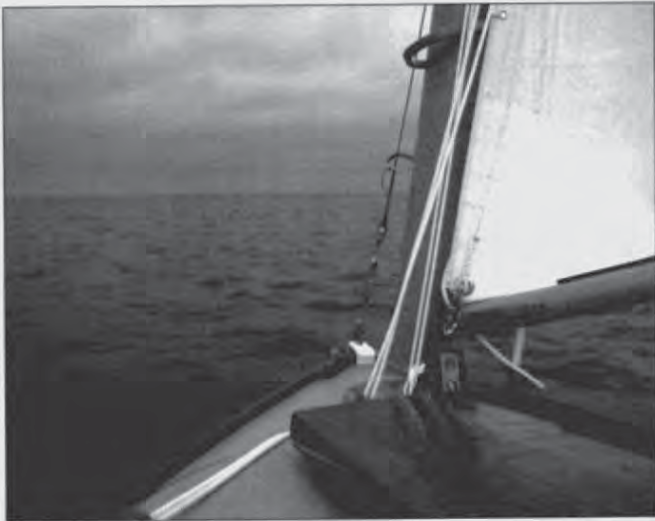
Note the color of the finish on the spars match. Also shown are the oak mast hoops and gooseneck fitting.
