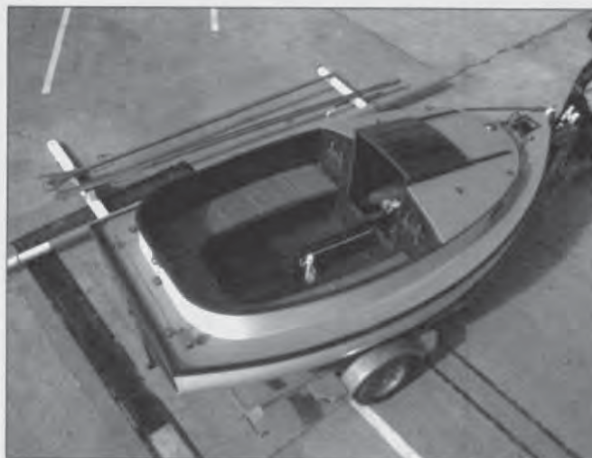
Layout of hardware on the new cat is shown here with the halyard fairleads and the ventilator cap on the cabin top, and mainsheet traveler and engine bracket fitting on the stern.
