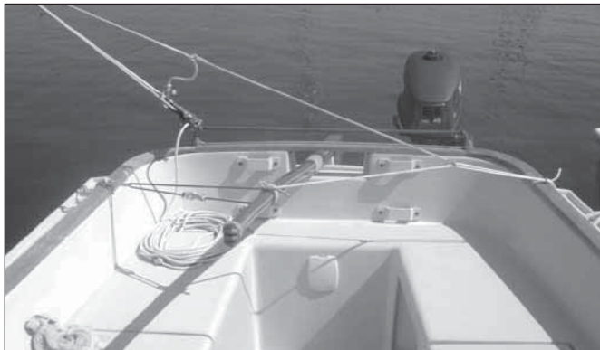
In a dead spot, or when the boat falls off too far the bungee pulls the tiller to leeward.
