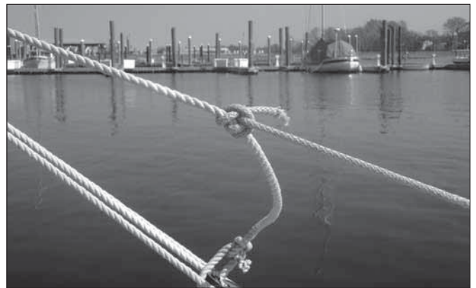
Rolling hitch on the mainsheet.
