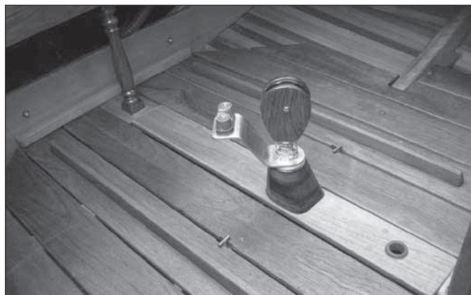
The main sheet cam cleat block installed on the cockpit sole to facilitate sailing with multiple crew particularly when the wind pipes up.
