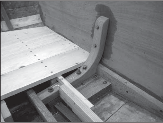
Floor is white cedar fastened with bronze.
