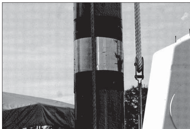
Aluminum flashing around mast hinge prevents parrel balls and sail hoops from snagging.
