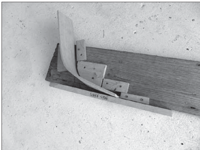
Figure 2: Bending jig. My 'workbench' is my garage floor.
