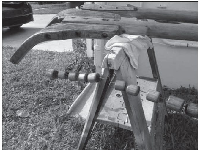
Figure 7: Epoxied and through bolted jaws – and new parrell beads made from 1 1/2 in. lengths of curtain rod dipped in varnish, drying in the sun.
