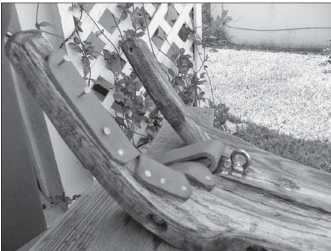
Figure 12: Tacking leather to jaws, tumbler is leathered.
