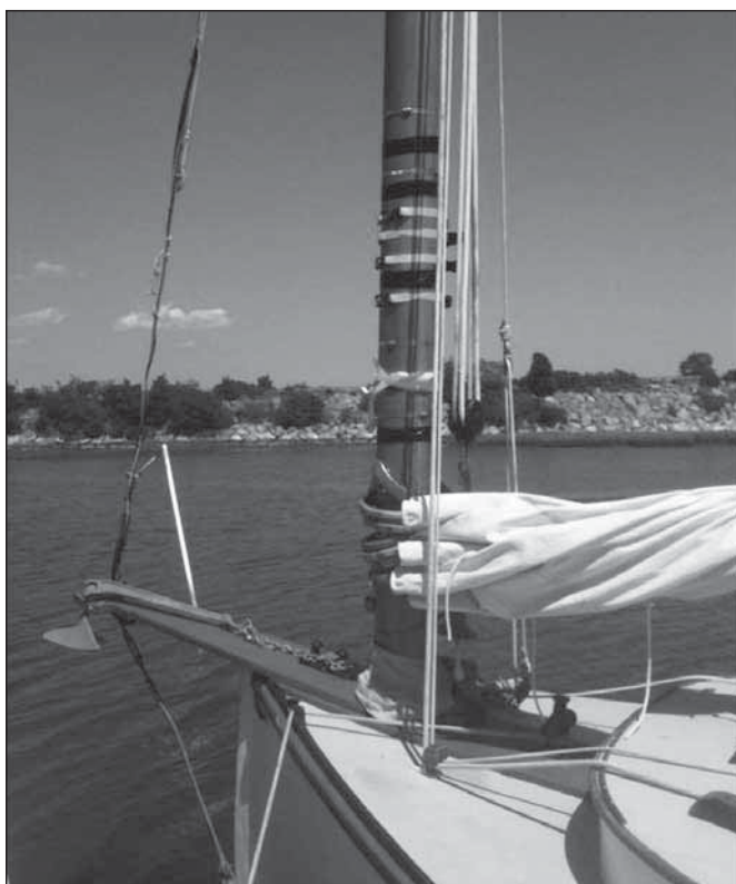
Buckrammer safe at Slight's wharf with numerous web and hose clamps holding things together.
