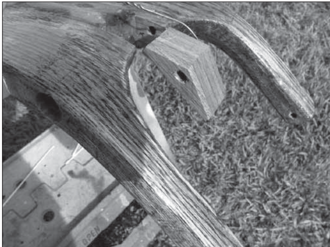
Figure 8: Gaff jaws with tumbler – not installed yet.
