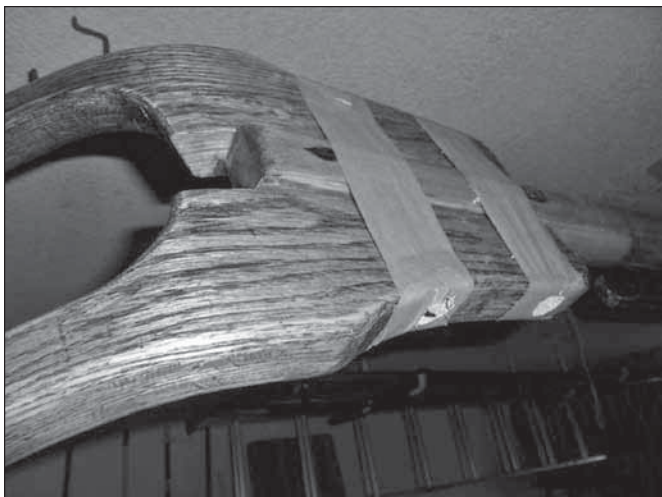
Figure 6: Countersunk holes are drilled on either side of epoxied jaws to allow for fastening to the gaff.
