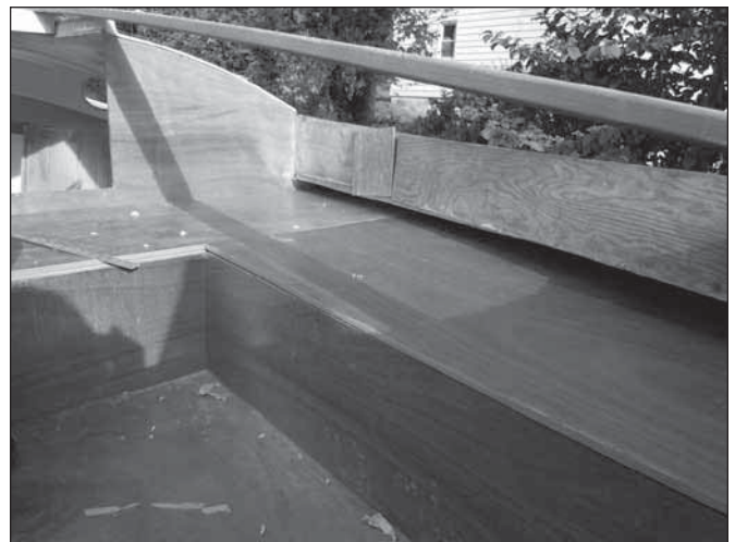
It's a beautiful golden color because I already coated the plywood in West Systems Epoxy.
