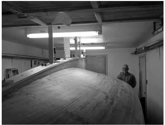
Installation of the final outer keel lamination December 3, 2012.
