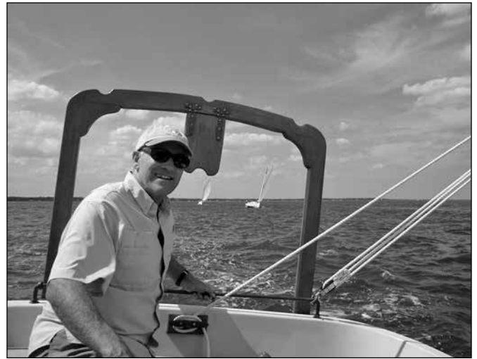
Gallows with hinged boom extension.
