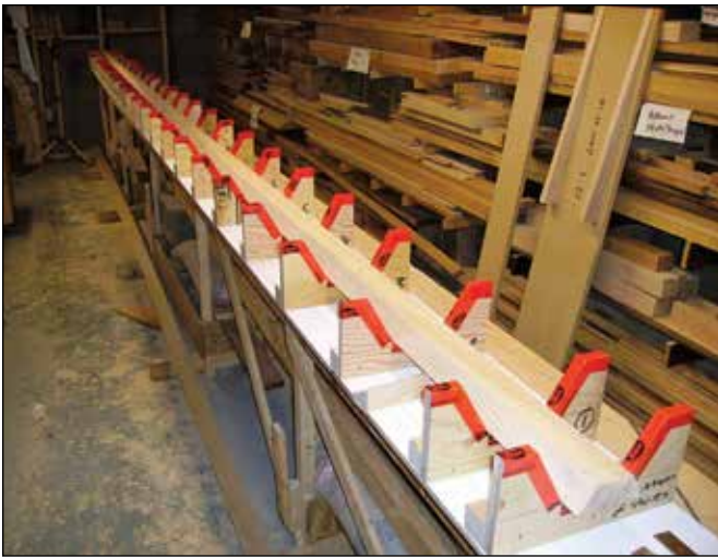
Mast assembly cradle.
