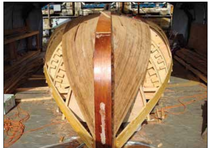
About 1/3rd planked, prior to tapering the stem.
