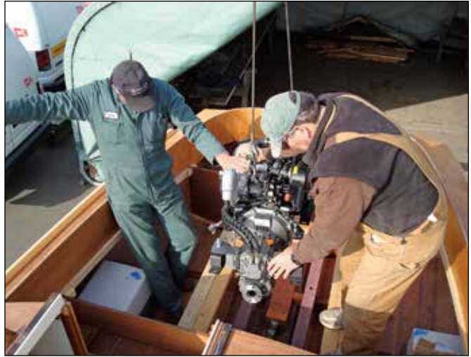
Roy Dunbar (right) placing the engine on the engine bed as Coastal Transportation's loading boss directs the crane.
