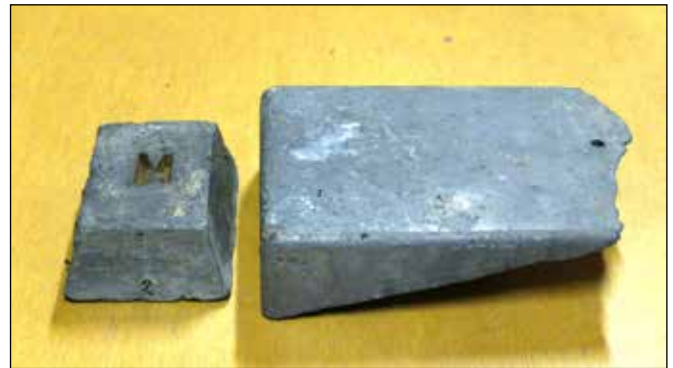
Original 20 lb. lead ballast pig and 50 lb. wedge, one of ten custom cast to make a level cabin sole 3 in. lower than the original. We used a power plane to refine the fit, bored a hole in each for a lifting loop, and used the gaff to get them aboard.
