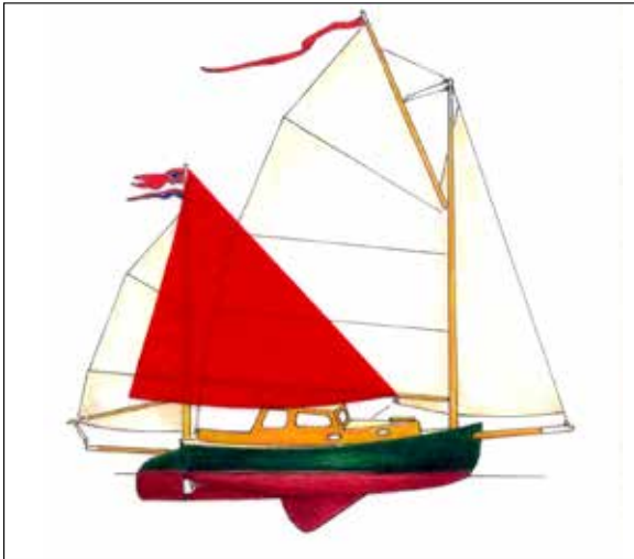
My wife Dee's preliminary sketch showing what we were aiming at. In the end the house was longer and lower, and the mizzen grew to a standing lugsail with a 10 foot yard.
