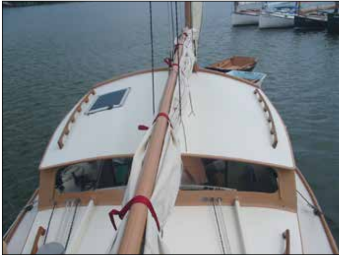
Halyards and reef pennants enter the doghouse to starboard; all except the luff reef line are controlled by sheet stoppers, and can be led to a winch. To port are the jib furling line, and lazy jack lift.
