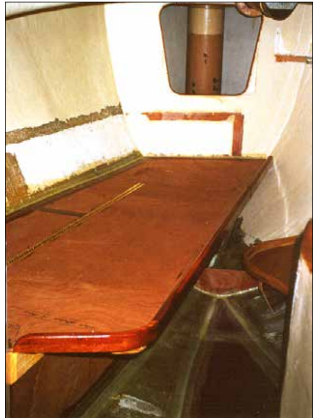
Nearly the best idea we had: A cantilevered bunk extension for the minimalist forward berth. The scars show where the original was tabbed to the hull and bulkhead.
