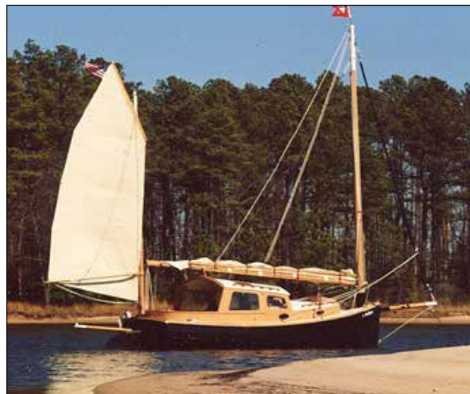
The Muskrat anchored in our favorite hidden cove, showing off her half-wishbone sprit boom.
