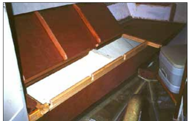
Our wider bunk would crowd the knees a little when using the portable toilet opposite unless raised as shown. With the cushion in place, it is held vertical by a lanyard.
