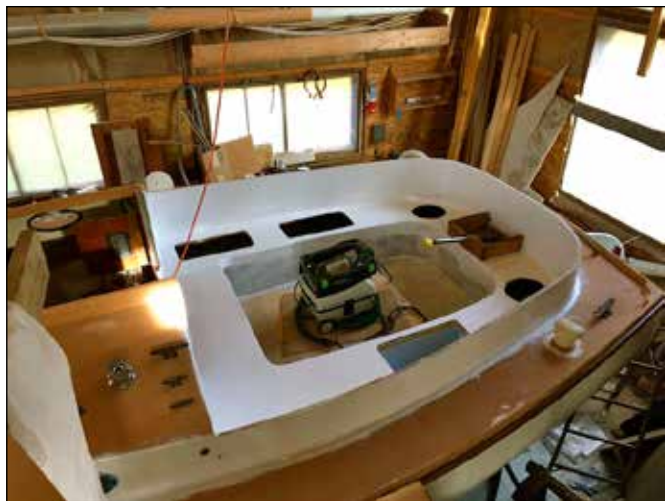
New cockpit glasswork complete with dry storage, freezer compartment, and foot extension for quarter berth under.
