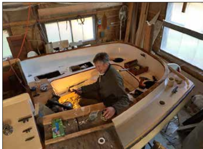
Paul Rollins (Rollins Boatshop, York ME) fitting new teak coaming and teak cockpit and cabin trim.
