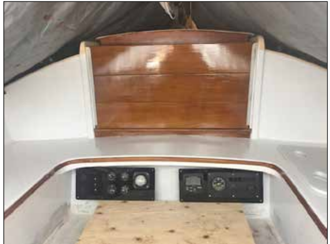
Cockpit ready to reconnect instrumentation under bridge deck, with teak wash boards and Beckson watertight hatches.
