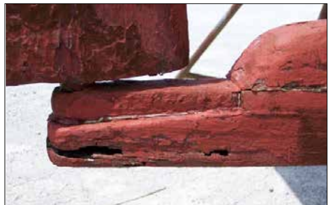
Bottom of the rudder post, the paint covers the worst of the worms' work.
