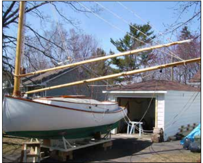
Mast stepped and rigging started.
