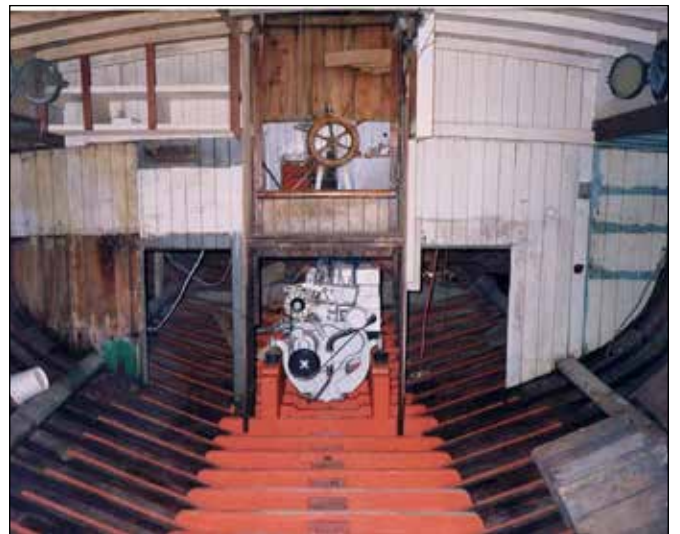
New Engine installed.
