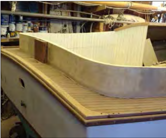
Cabin frame and roof and hatch. Anyone want to venture a guess at how many bungs are on the hull?
