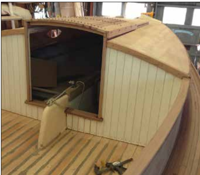
Cabin frame and roof and hatch. Anyone want to venture a guess at how many bungs are on the hull?
