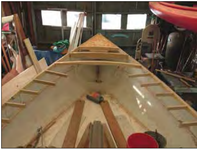
Deck beams and new floor.
