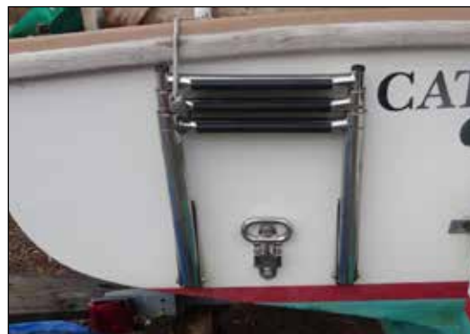
Transom ladder folded. Folding step makes boarding after a swim much easier.
