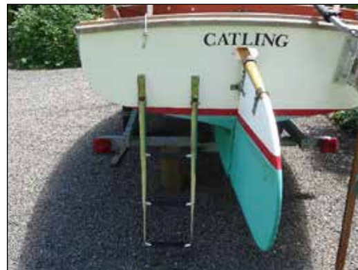
Transom ladder extended. Note distance from the top rung to the afterdeck.
