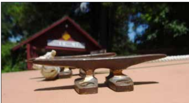
A jam-cleat cleat after filing.
