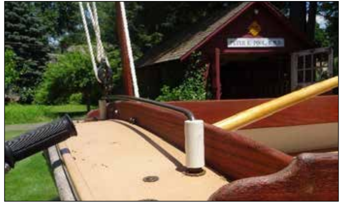
Traveler with one inch PVC pipe installed port and starboard.
