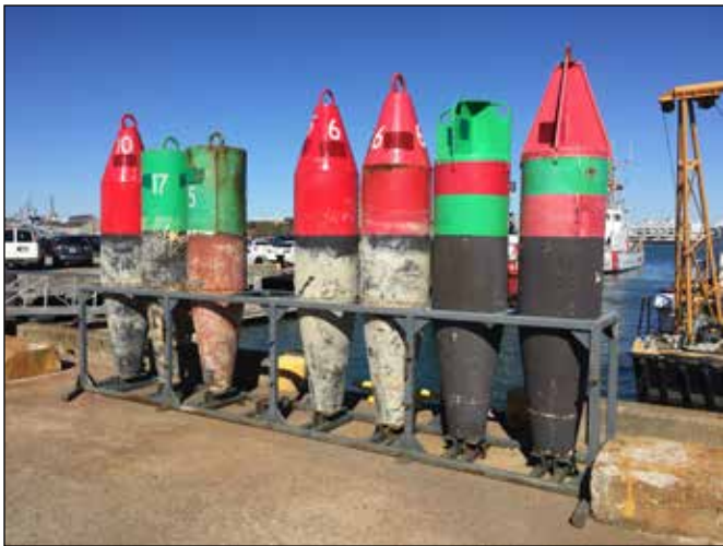
A rack of 5th class aids at Base Boston. The can and nun on the far right are radar reflecting, the others are not.
