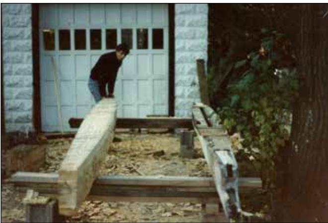
Beginning the new keel with the old one beside it.
