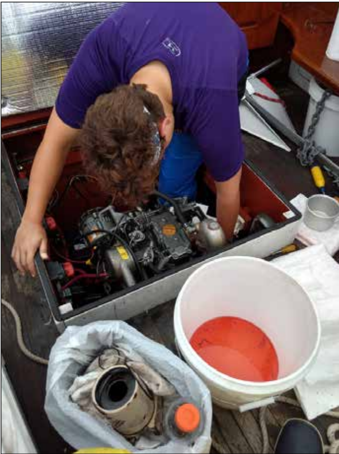
Replacing filters and bleeding fuel lines.
