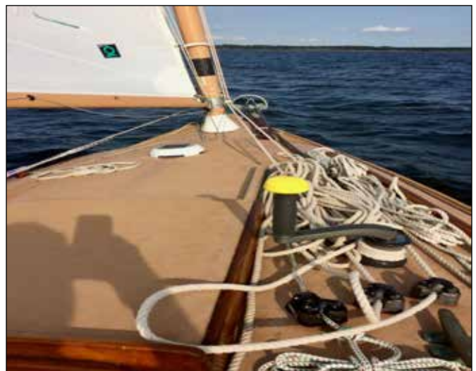
The foredeck. Note the anchor board forward and Lewmar winch in the foreground.
