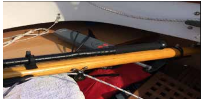
Tiller with line for securing in port. I use this same line to hold the tiller briefly while underway.
