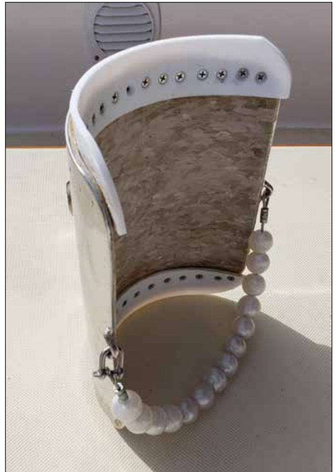
Improved gaff saddle – Teflon guards. Note the small shackle on the left end of the parrel.
