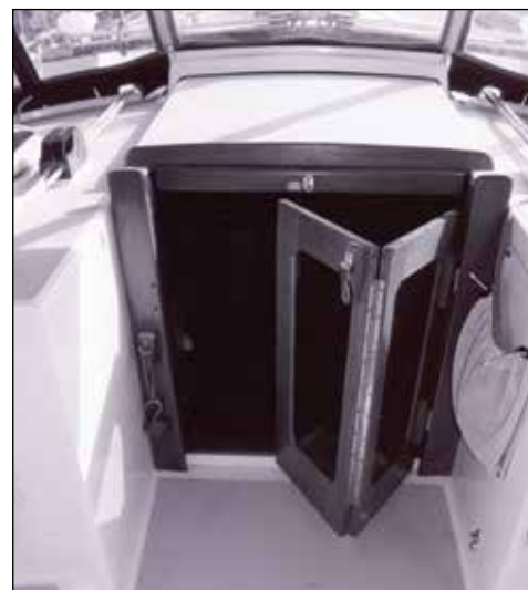
Bifold door with Lexan panels.
