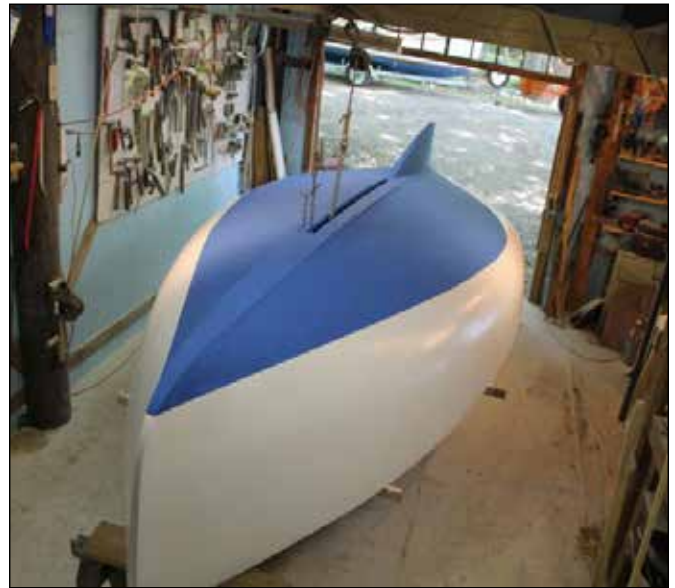
Figure 8. After gelcoat and bottom painting.
