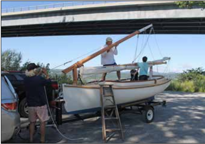
Figure 21. Raising the mast.
