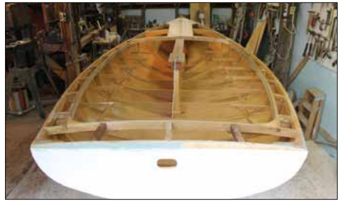
Figure 11. Ready for sole, seats, and deck.
