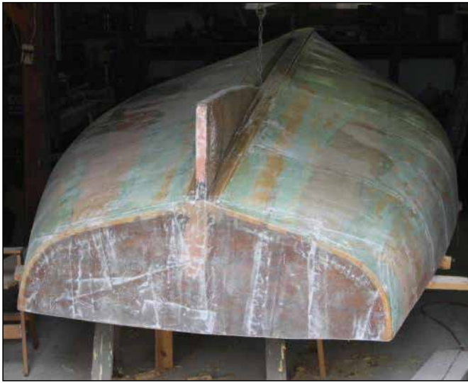
Figure 6. The hull 'glossed and ready for fairing.
