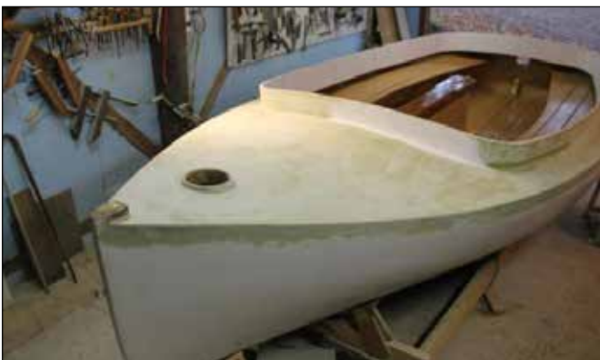
The deck structures roughly fiberglassed.
