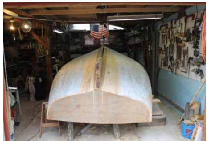
Figure 5. The planking complete.
