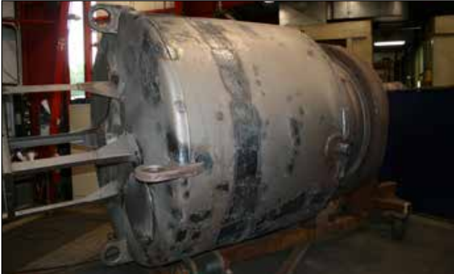
A buoy after welding. Note the band around the upper portion of the vessel approximately at the waterline—a common location of rusting/ pitting.
