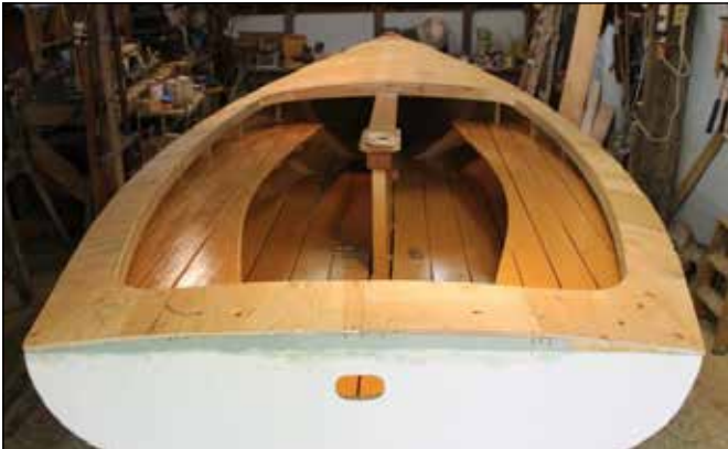
Figure 13. The deck roughly installed.
