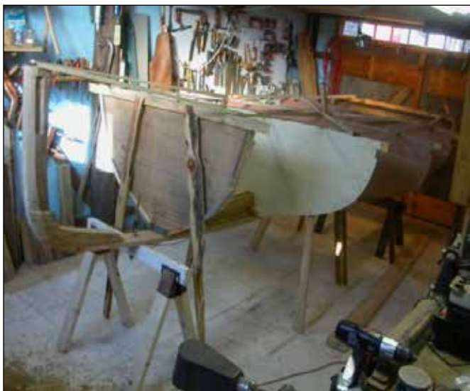
Figure 3. The station moulds in place.
