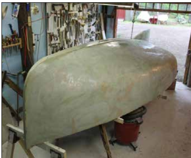
Figure 7. The hull after fairing and sealing.
