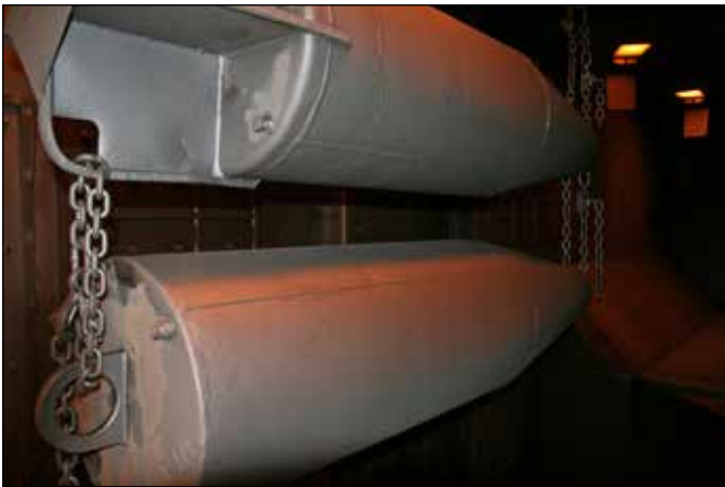
A buoy after sandblasting.
