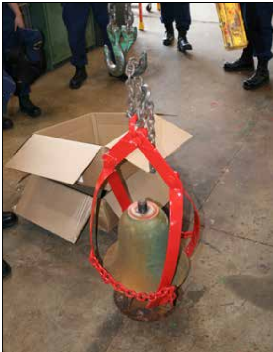
The bridle for lifting a bell onto an aid.
