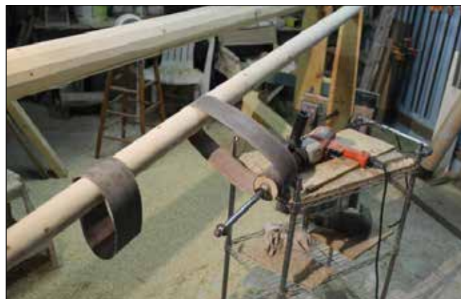
Figure 19. Shaping the mast and boom on progress on the spar sanding tool I made.
