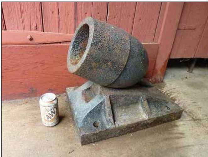
The Manby Mortar used for sending lines to stricken vessels. The soda can is there to provide a size reference.
