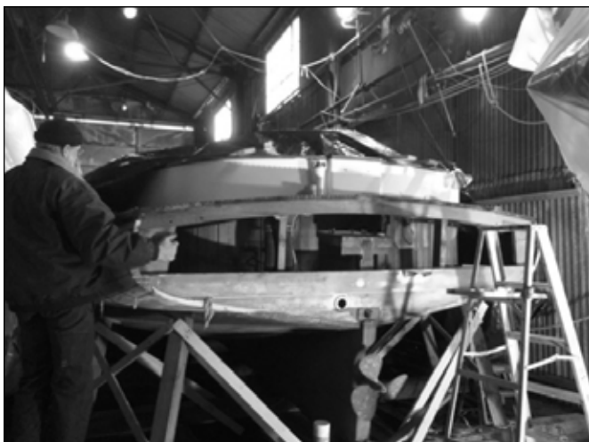
Twenty-two years after restoration in 1998, the 1916 catboat Victor had developed rot in two oak transom planks and part of the aft frame. These are being replaced by Tom Wells in Greenport, New York.
