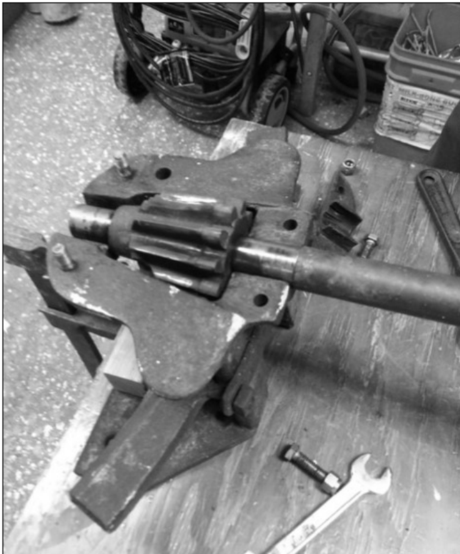
The original steering gear from The Victor . Note broken teeth in the pinion gear. Edson Marine located a replacement. The old, existing pinion gear is cast iron. The new one will be nickel bronze. Fortunately, the base shown here was in very good condition.
