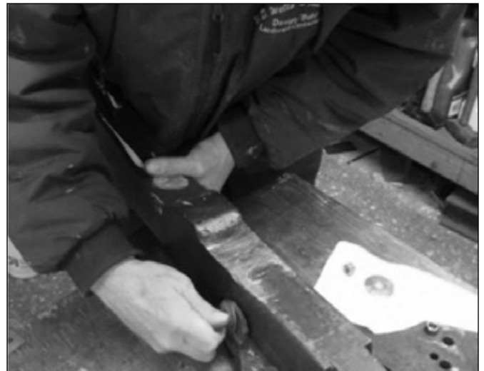
Where the tiller bolts onto the rack there was a problem because of the lip on the rack was rusted and thin. Tom used epoxy with carbon fiber to build it up for a tighter fit
