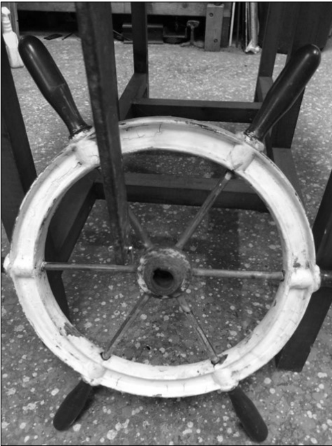
The original, the Edson people say rare, bronze steering wheel. This wheel will be refurbished.
