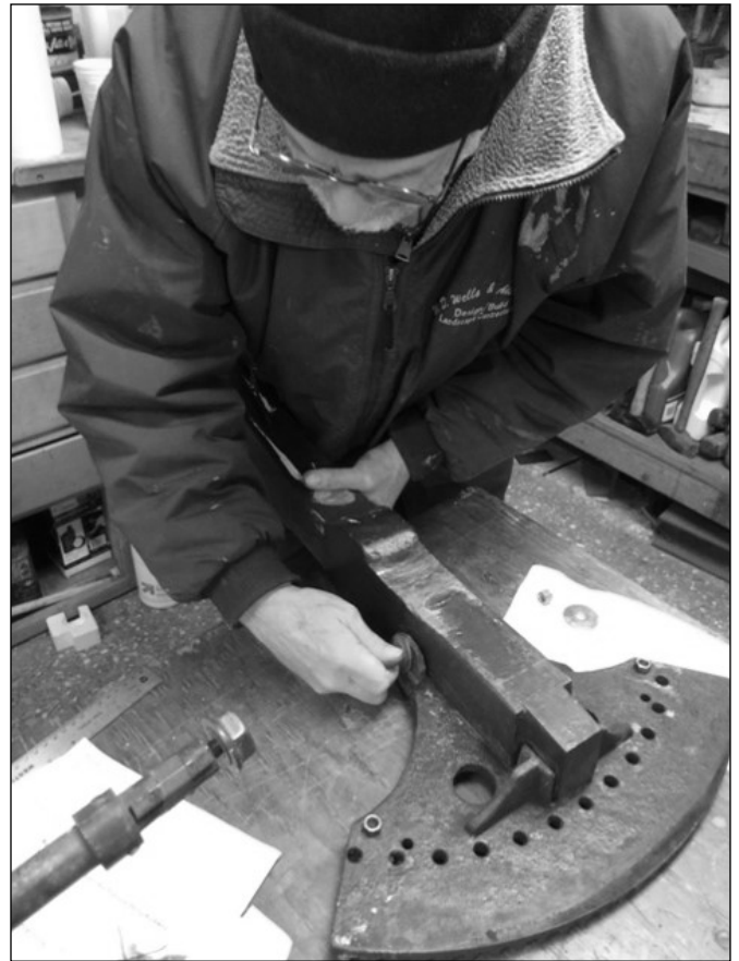
Shipwright Tom Wells fitting bolt through oak tiller on cast iron rack. The original Edson steering gear is still in service.
