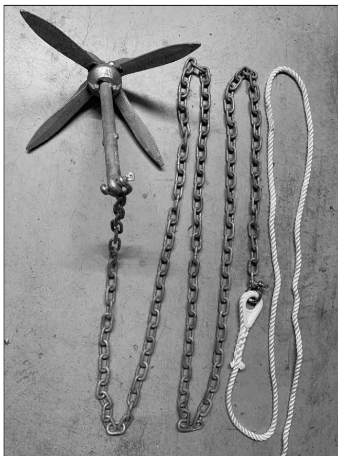
Figure 1. An anchoring system: anchor, chain and line.
