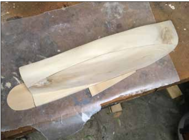
The half-hull after shaping, with the rudder and centerboard installed...
