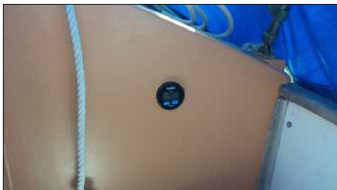
Figure 5. Depth finder display installed – outside.
