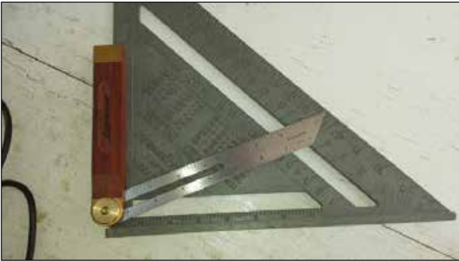
Figure 2. Measuring the deadrise.
