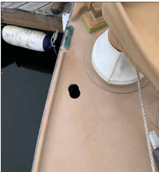
The hawse pipe hole in the deck.
