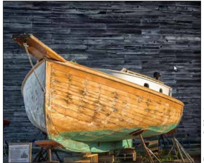
Figure 1. Once "wooded" the boat revealed what fasteners needed replacement.
