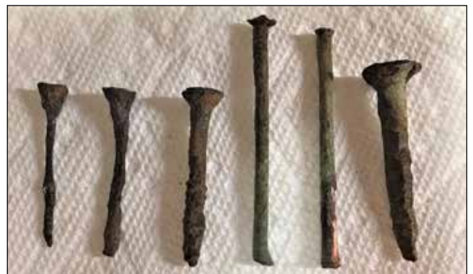
Figure 2. Many of the fasteners were "shadows of their former selves."
