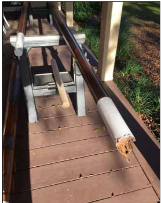
The rotted end of Betty Jane's Boom.
