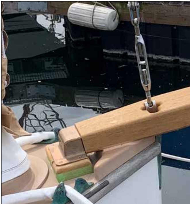
The bowsprit in place.
