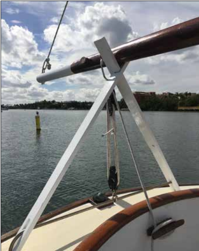
The new boom crutch in place.
