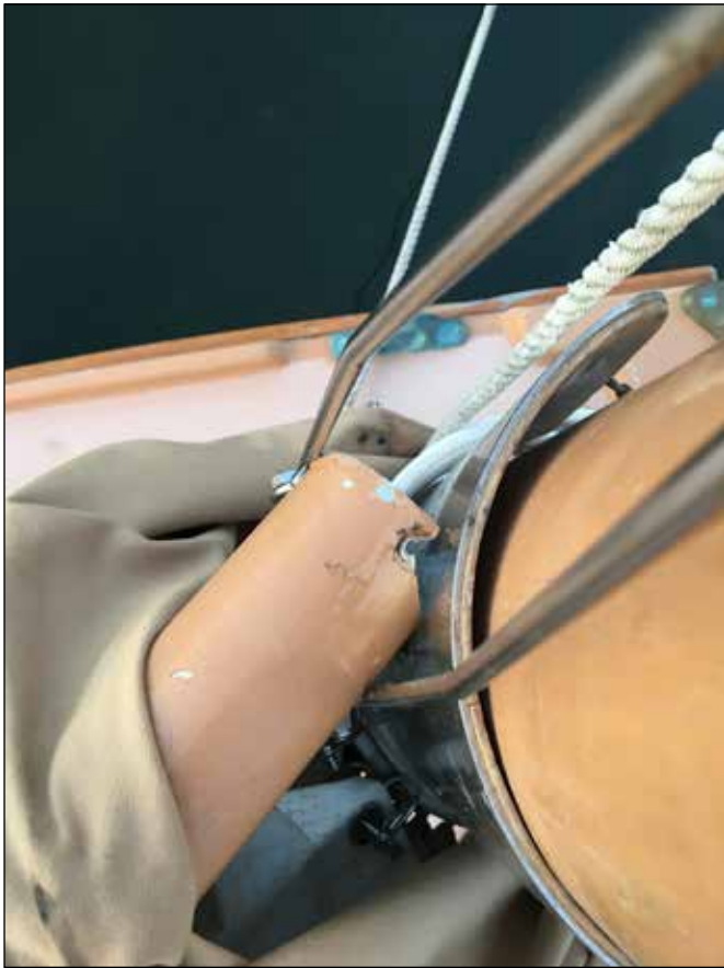
Broken gooseneck Block Island.
