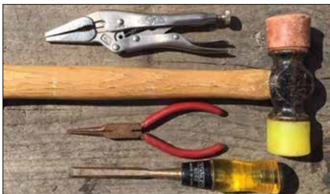
Figure 3. Five simple hand tools and an electric drill make quick work of removing failed fasteners.
