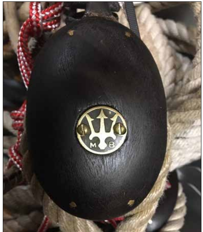
Figure 16. Virtually all of Marvel ’s rigging runs through restored Merriman Brothers blocks.
