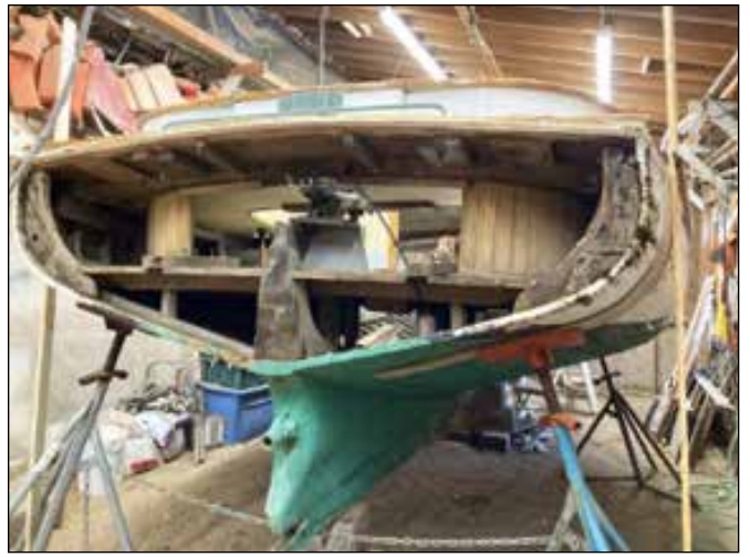
The transom under repair.
