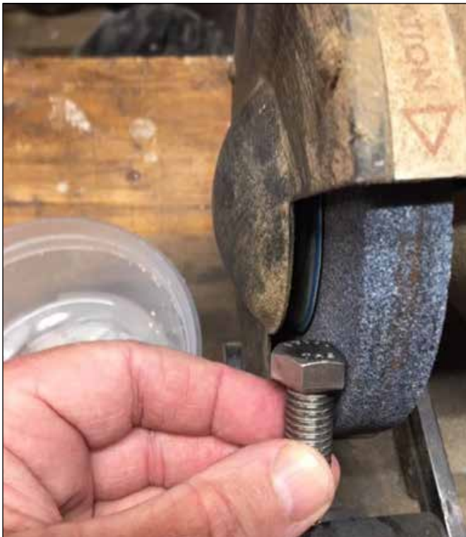
Figure 12. By grinding off a bit of its mounting bolt, the starter re-install went smoothly.
