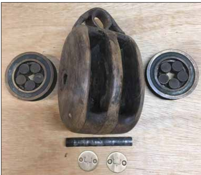
Figure 17. The ingenious design of Merriman blocks allows them to be readily restored.
