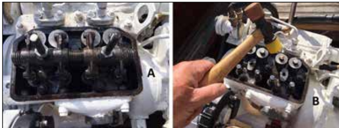
Figure 4: A simple procedure tests to see if an old engine’s valves are stuck.
