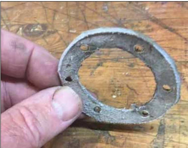
Figure 6. A hand-made Elk-skin gasket would restore the seawater pump with style.
