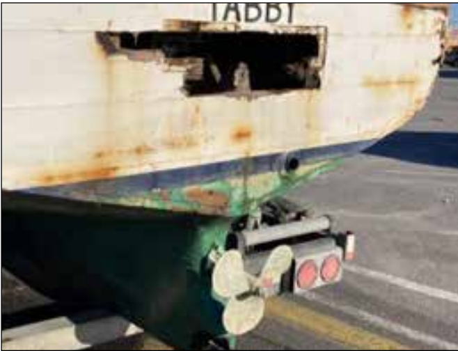
The hole in the transom where the quadrant pulled through.
