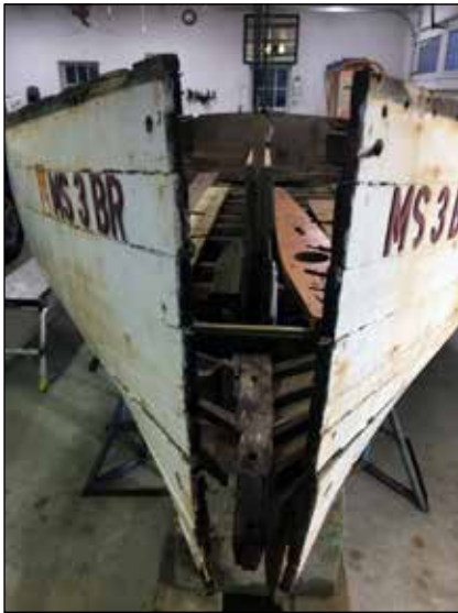
The stem, forefoot and mast step were one of the first things to go.
