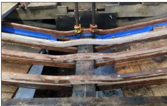
The ribs were fitted into pockets cut into the keel. In Addition, Manuel Swartz Roberts connected the ribs together with a steam bent piece of oak that rode over the keel.
