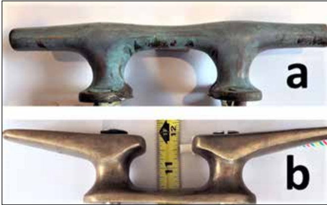
Figure 6: A catboat's aft cleat (b) allows skippers to quickly lock and release the main sheet.
