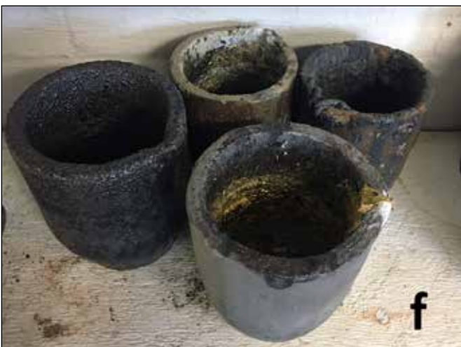
An appropriate crucible is selected (Figure 4f), loaded with bronze ingots.
