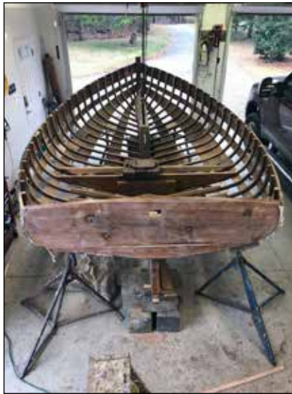
The framework for the planking completed.
