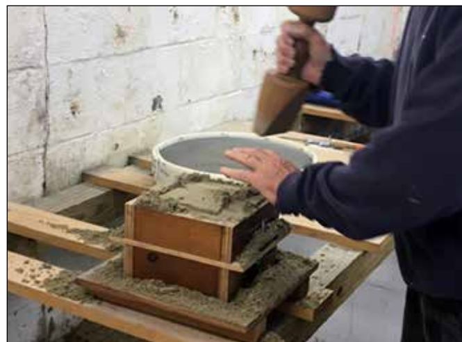
The flask is then tipped over. Pour forms are inserted and the bottom half of the assembly was filled with the pounded sand/clay mix. (Figure 4c)
