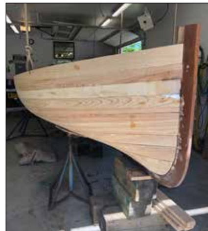
The planking installed, bunged and faired.
