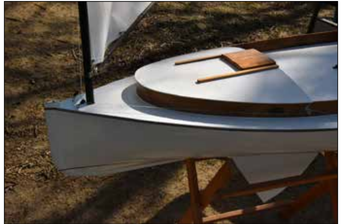
The foredeck and gooseneck. Note the halyard details.
