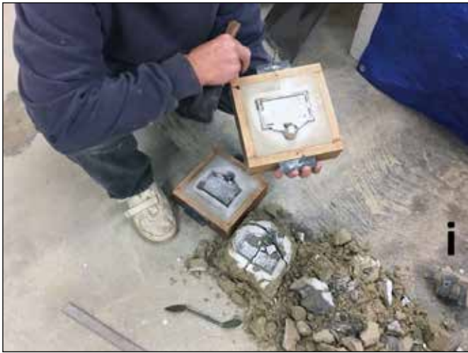
After about four hours of cooling, the reproduction was ready to be liberated from the flask. Using a special tool, my friend knocked away the sand/clay mix to reveal the reproduced plaque. (Figure 4i)
