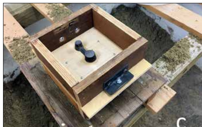
The flask is then tipped over. Pour forms are inserted and the bottom half of the assembly was filled with the pounded sand/clay mix. (Figure 4c)
