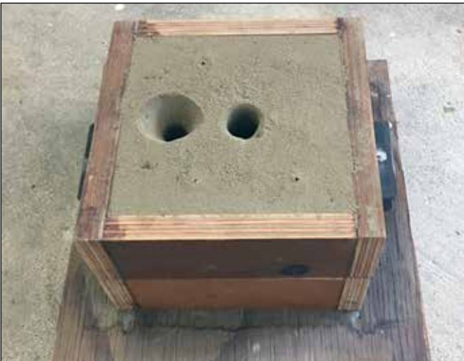
The flask is then reassembled and inverted with the pour holes on top. (Figure 4e)
