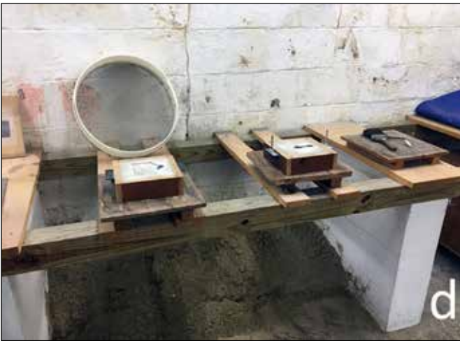
The two halves of the flask are then separated, and the original plaque is carefully removed. This reveals the impression of the original plaque which will serve as the casting mold. (Figure 4d)
