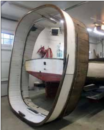
The entire cockpit coaming was able to be removed in one piece. This later proved to be a great aid in replicating the new coaming.
