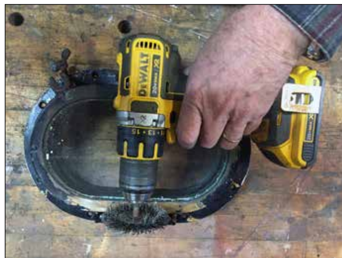
Figure 18: Lots of wire brushed elbow grease began the process of porthole restoration.
