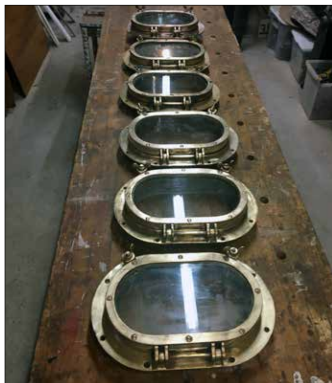
Figure 19: The refurbished and restored large portholes are ready to return to service.
