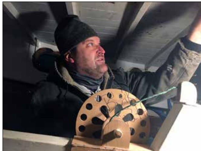
Figure 11: Master boatwright George Schuld fitting his wooden winch prototype undercover.
