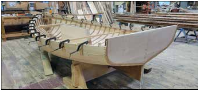
Installing sheer clamps – Beetle 14.
