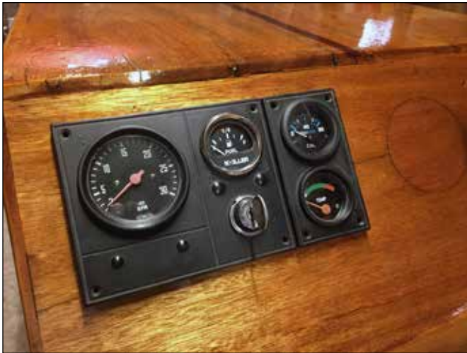
Figure 20: With new gauges installed, the restored engine cover is ready for reinstallation.
