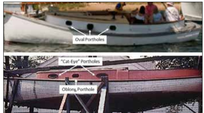
Figure 9: Comparisons of cabin and porthole modifications.
