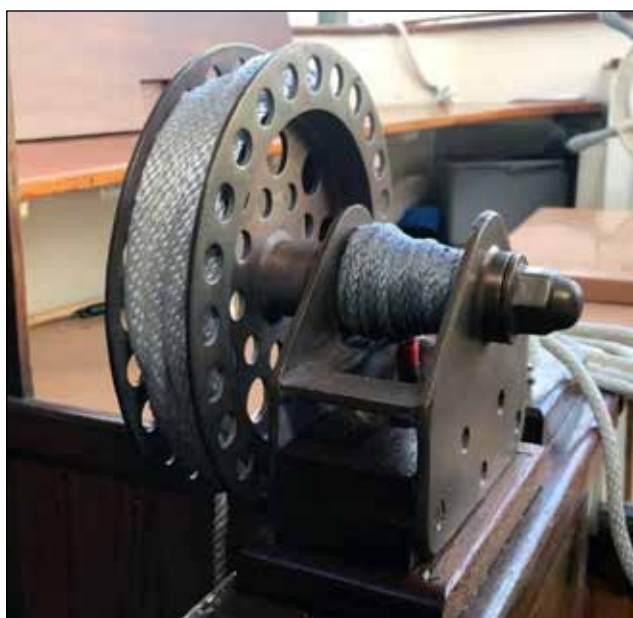
Figure 10: Racing style, antique centerboard winch aboard the catboat Fairweather .
