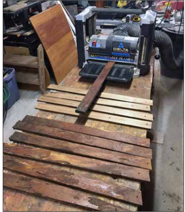
Figure 15: Teak salvaged from the rotted deck section and elsewhere was recycled for the hatch.
