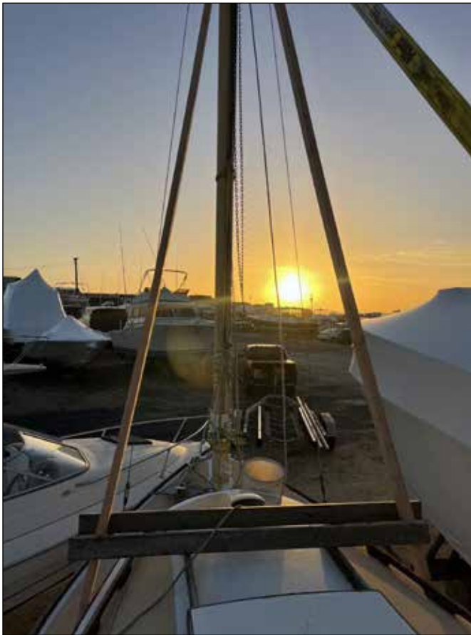
The A-frame and mast removal setup, before things went sideways....
