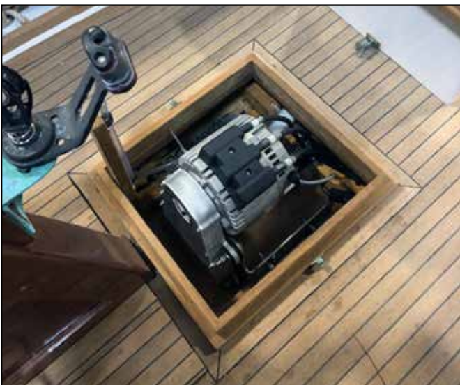
OceanVolt's shaft driven electric motor installed in a sixteen foot Arey's Pond Lynx
