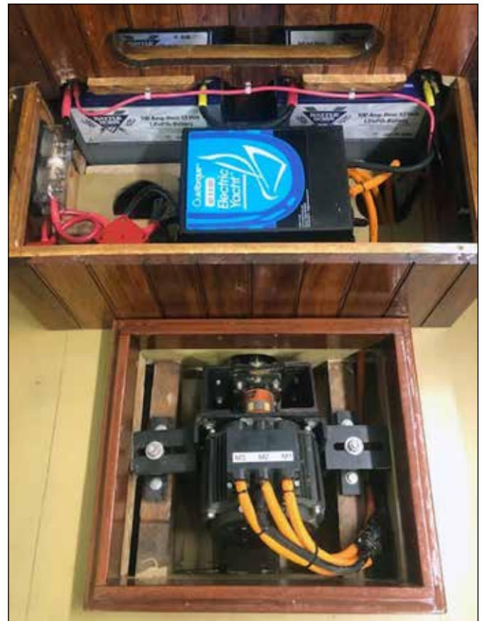
Electric Yacht's shaft driven electric motor installed in fifteen foot wood catboat.
