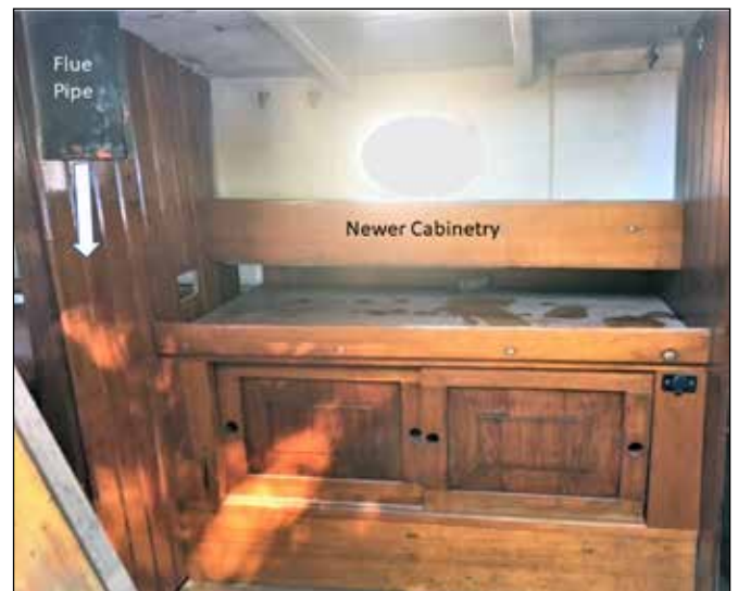
With the flue pipe misaligned, there was no place to mount her Shipmate #1 stove.
