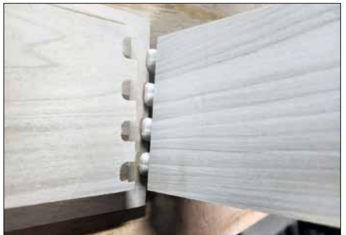
Figure 2. The pinboard and tailboard of the prototype drawer made from poplar.
