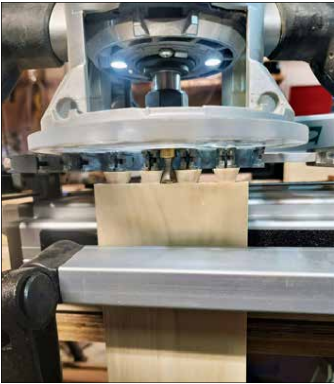
Figure 5. Cutting the vertically-clamped tailboards (drawer sides).
