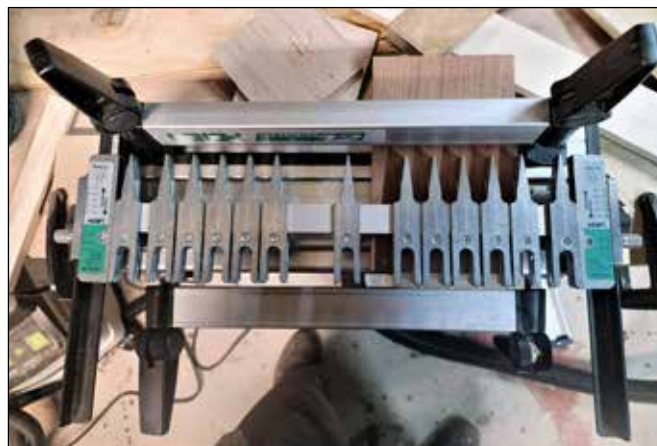
Figure 4. Adjustable Fingers Form the Comb on the Leigh Super 12 Dovetail Jig. They Can Be Adjusted into Symmetrical Patterns
