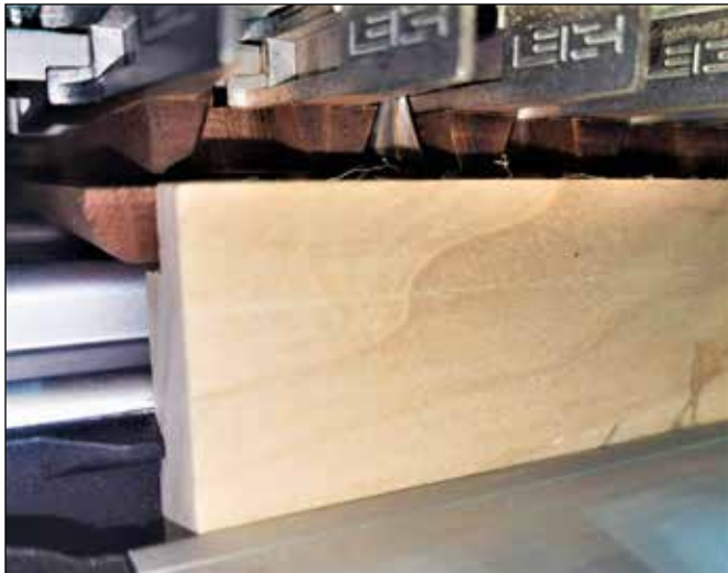
Figure 7. A rabbeted half-blind pinboard with a rabbeted scrap board in front of it.
