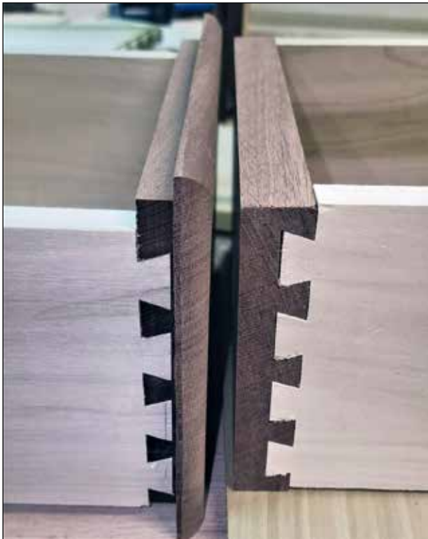
Figure 1. Rabbeted half-blind and half blind drawers. The dark sapele wood is the front pinboard, the white poplar, the tailboard.
