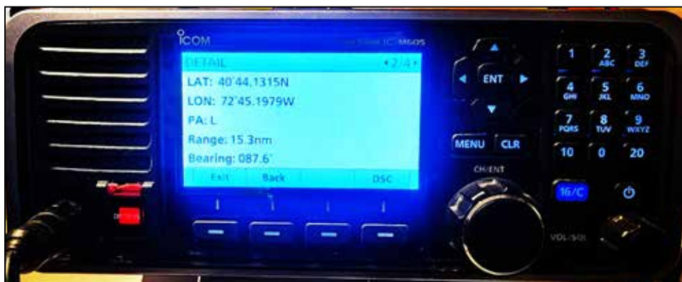
Screen 2 gives the GPS location, range and bearing to "M."
