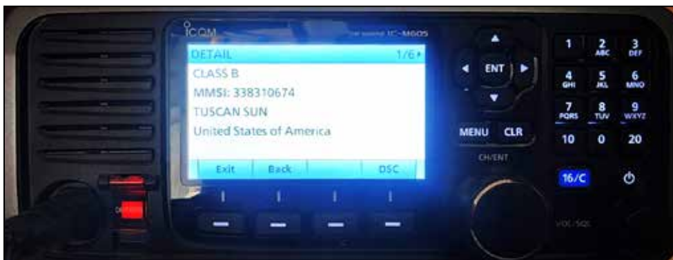
By pressing the button under DSC, a non-distress call can be made to the Tuscan Sun .
