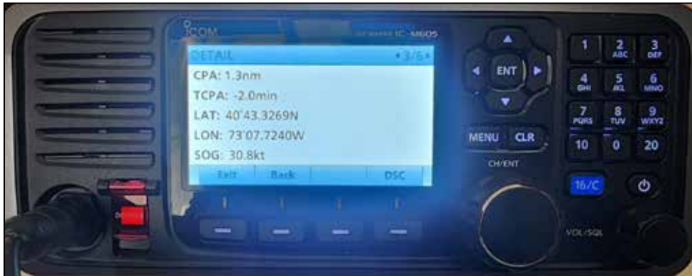
A VHF Radio with AIS can keep track of CPA and TCPA information.
