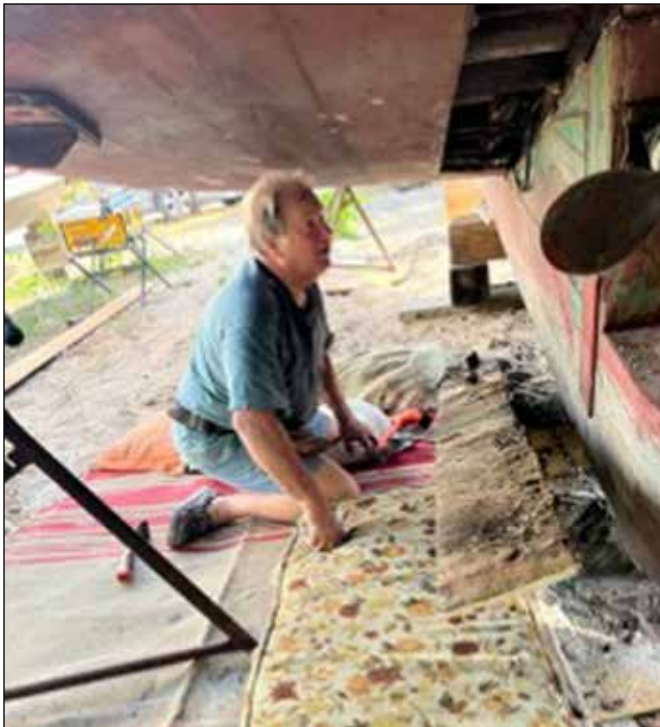
Bob Luckraft removes her port garboard to inspect the stop waters.
