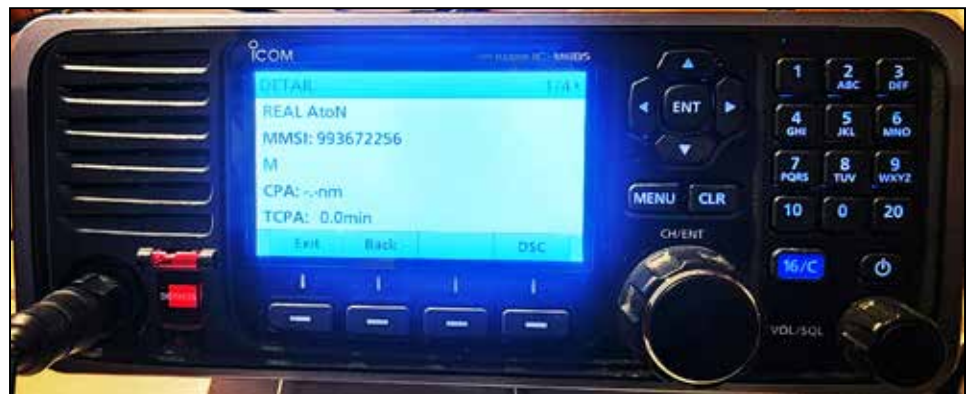
Screen 1 identifies "M" as an aid to navigation—the Moriches mid-channel buoy.
